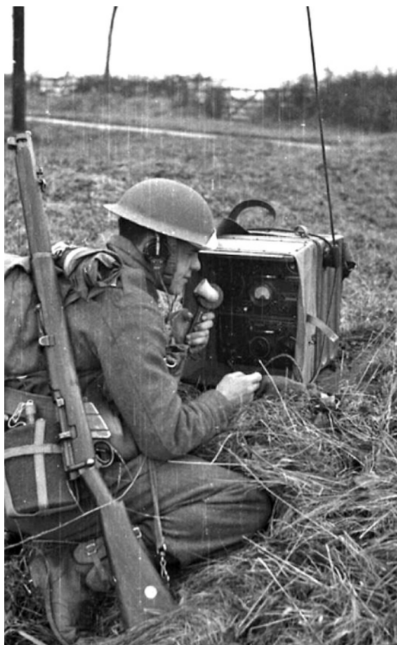
Two rare photographs of Wireless Set No. 8 being used during training of Czechs in exile in the early part of World War 2.
